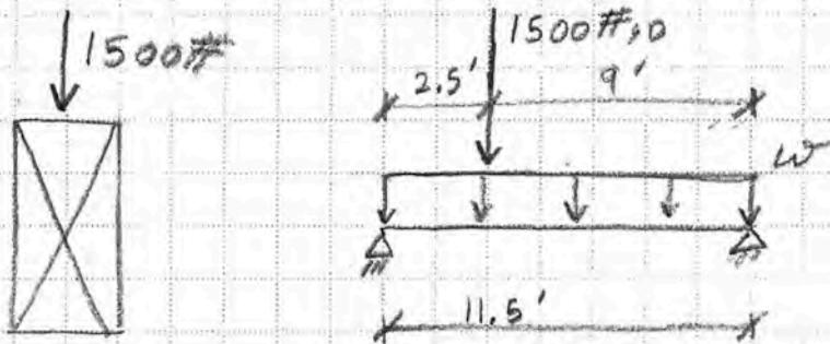
$$w = [60 \text{ psf}, L + 8 \text{ psf}, D] * 0.72 \text{ ft} = 43.2 \text{ PIF}, L + 5.8 \text{ PIF}, D \\ = 49 \text{ PIF}$$
