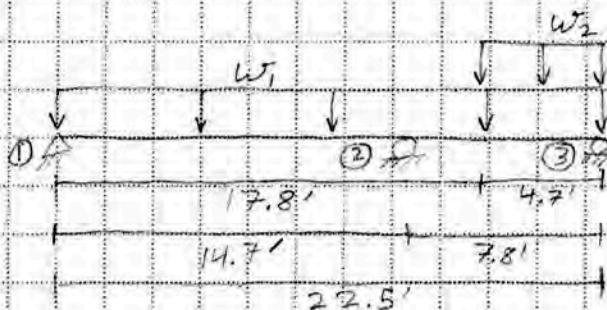
$$W_1 = [60 \text{ psf}_{\text{lb}} + 8 \text{ psf}_{\text{D}}] * (8.6'/2) = 292 \text{ PIF}$$
