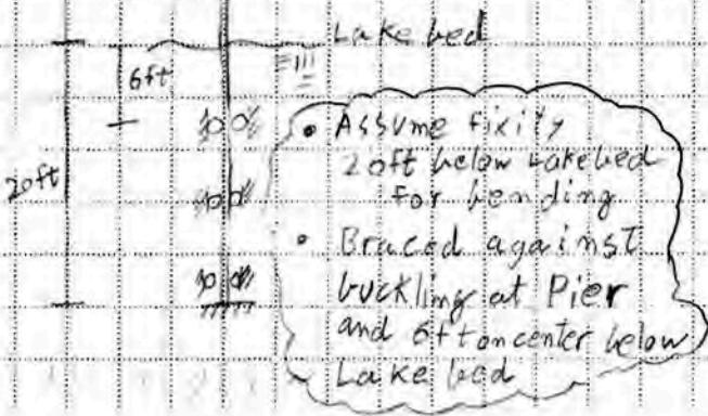
$$\begin{aligned} D &= 1164 \text{ #} \\ L &= 348 \text{ #} \end{aligned}$$
