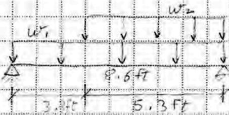
$$w_1 = [30 \text{ psf} + 8 \text{ psf}] * (12.5 \text{ ft} / 2) = 425 \text{ plf}$$
